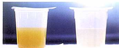
Comparison of: (left) wastewater treated with DAF system, and (right) wastewater treated with ASH system.
